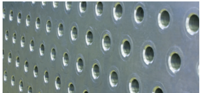
Tubeplate with smoothly rolled-in tubes.
