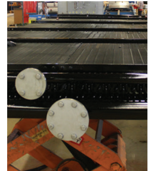
E-coating, with C5 classification, makes the cooler corrosion resistant for over 15 years.
