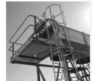
Railing, ladder & maintenance platform.
