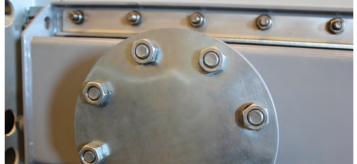
Headers made of anti-corrosion coated steel.
