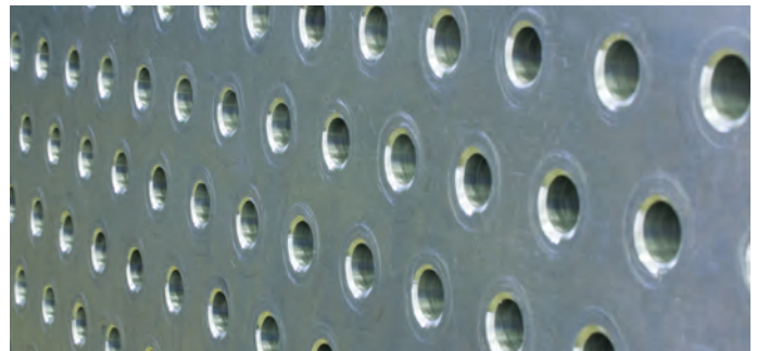
Tubeplate with smoothly rolled-in tubes.
