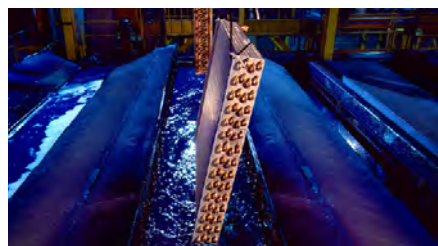
ElectroFin® E-coat process with C5-M and C5-I.
