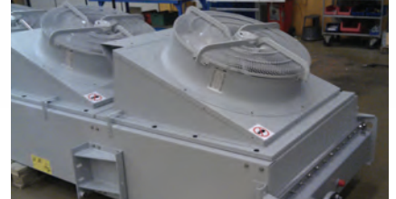
Transformer oil cooler with angled fan sections . Designed for efficient and directed evacuation of hot exhaust air.
