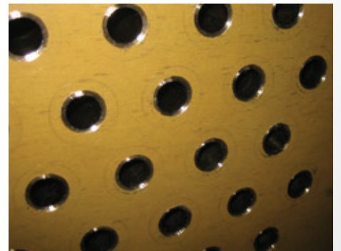
Tube plate with smooth rolled tubes.
