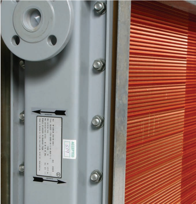
Single tube cooler with copper fins resist saline environment very well.
