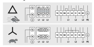
For other connections refer to the diagram printed on the inside of the motor-fan box.
