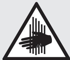
The operator at the stages of use and cleaning must be careful of the fins as they are sharp.
