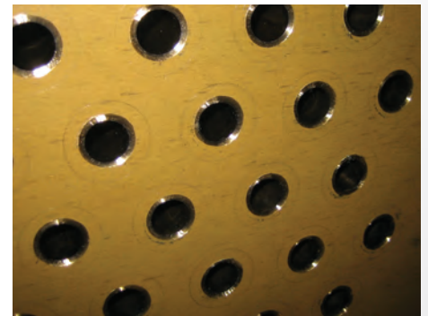
Tube plate with smooth rolled tubes.
