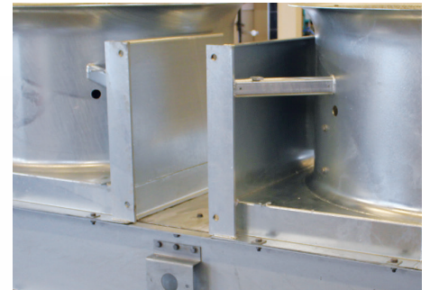
When two fan units are used, the fans are separated by a partition wall to give incremental power regulation.
